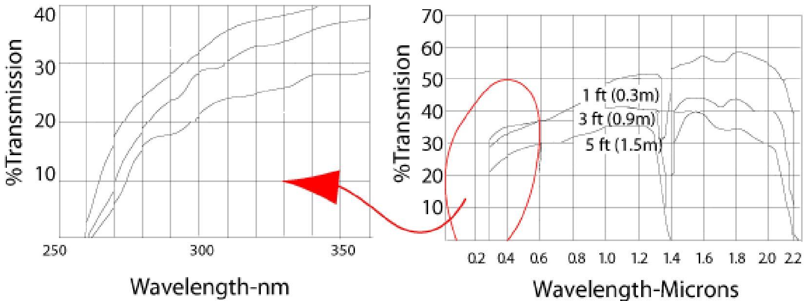
Characteristic spectral response of quartz optical fibre light guides taken from Edmund Optics online catalogue:
