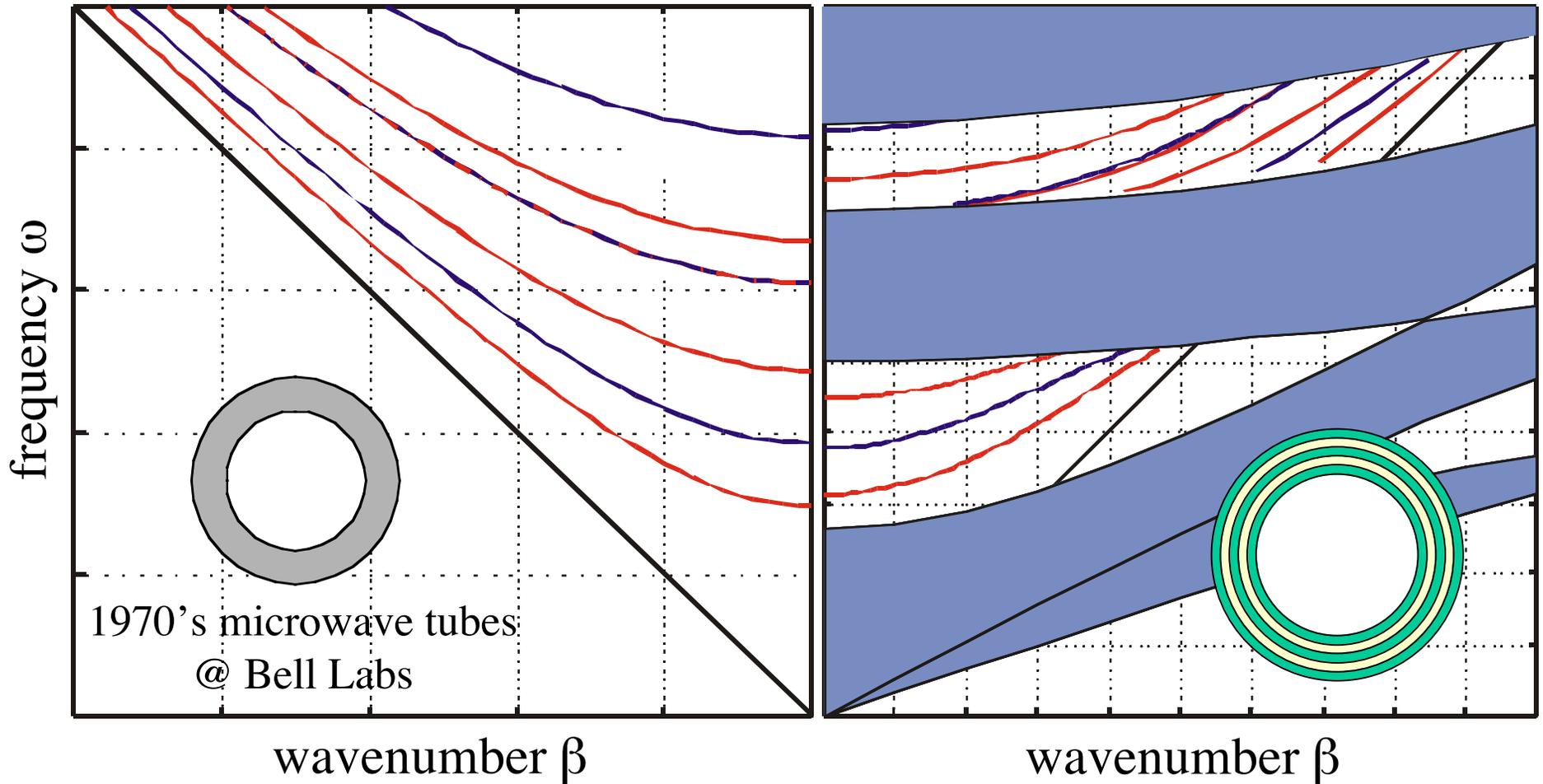
modes are **directly analogous** to those in hollow metal waveguide
