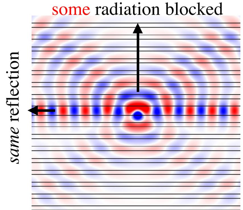
...with Si/SiO<sub>2</sub> Bragg mirrors (1D gap)
