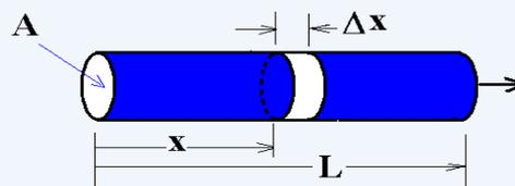
We assume the rod is of a homogeneous material and the surface of the rod is insulated so that heat flows only in the  $x$ -direction. Conservation of energy requires that the rate of change of heat energy associated with the volume element must equal the rate of heat energy flowing across the ends of the volume element plus any heat energy produced inside the element of volume. The physical properties of the rod are represented by the quantities:
