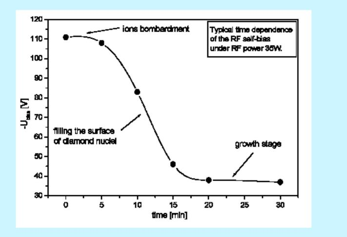
• the BEN method was used during the whole growth of the diamond film because of continuous diamond crystals nucleation leading to the deposition of UNCD films
