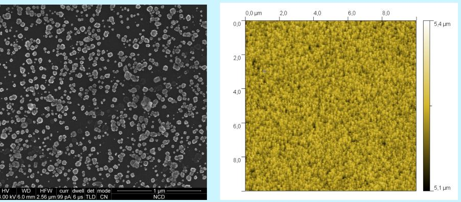
Sample S2: termination of surface nucleation and subsequent three-dimensional growth of individual crystallites
